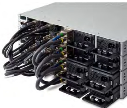
Figure 6. Cisco Catalyst 9300 Series StackPower
