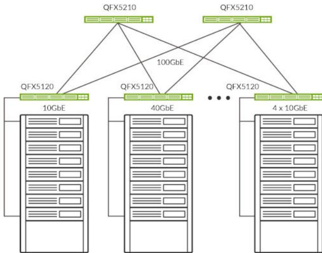
Figure 2: QFX5120 and QFX5210 leaf-spine deployment with distributed gateway
