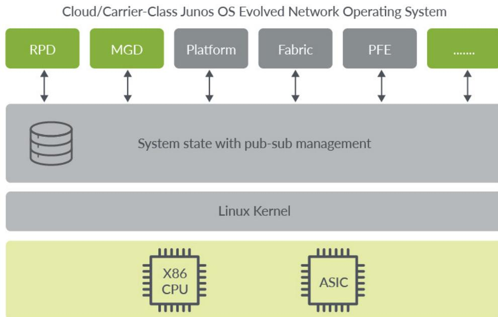
Figure 4: Cloud/Carrier-Class Junos OS Evolved Network Operating System
