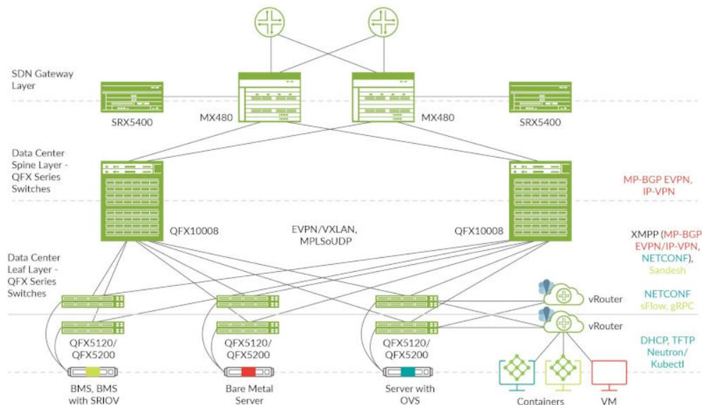
Figure 3: Contrail Enterprise Multicloud as a fabric management and SDN overlay for data center infrastructure
